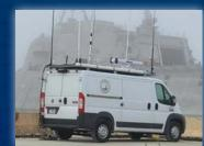
Mobile test vans are also available to support testing of vessels in shipyards and other locations away from the Fleet Concentration Area ranges.
